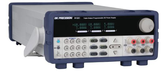
The 913OC Series triple output linear programmable DC power supplies feature isolated outputs that can be adjusted independently or combined in series or parallel to output higher voltage or current. Additionally, these supplies can operate in tracking mode with user-configurable ratios between channels.
